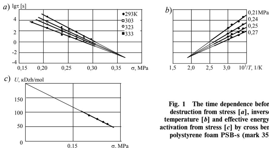
**Fig. 1 The time dependence before destruction from stress [a], inverse temperature [b] and effective energy of activation from stress [c] by cross bend of polystyrene foam PSB-s (mark 35)**
