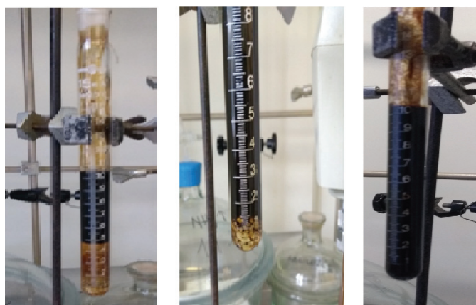
Fig. 3. Emulsion samples with different pH (pH = 7, 04 and 02) after 20 minutes, 90 minutes and more than eight weeks respectively (from left to the right)
